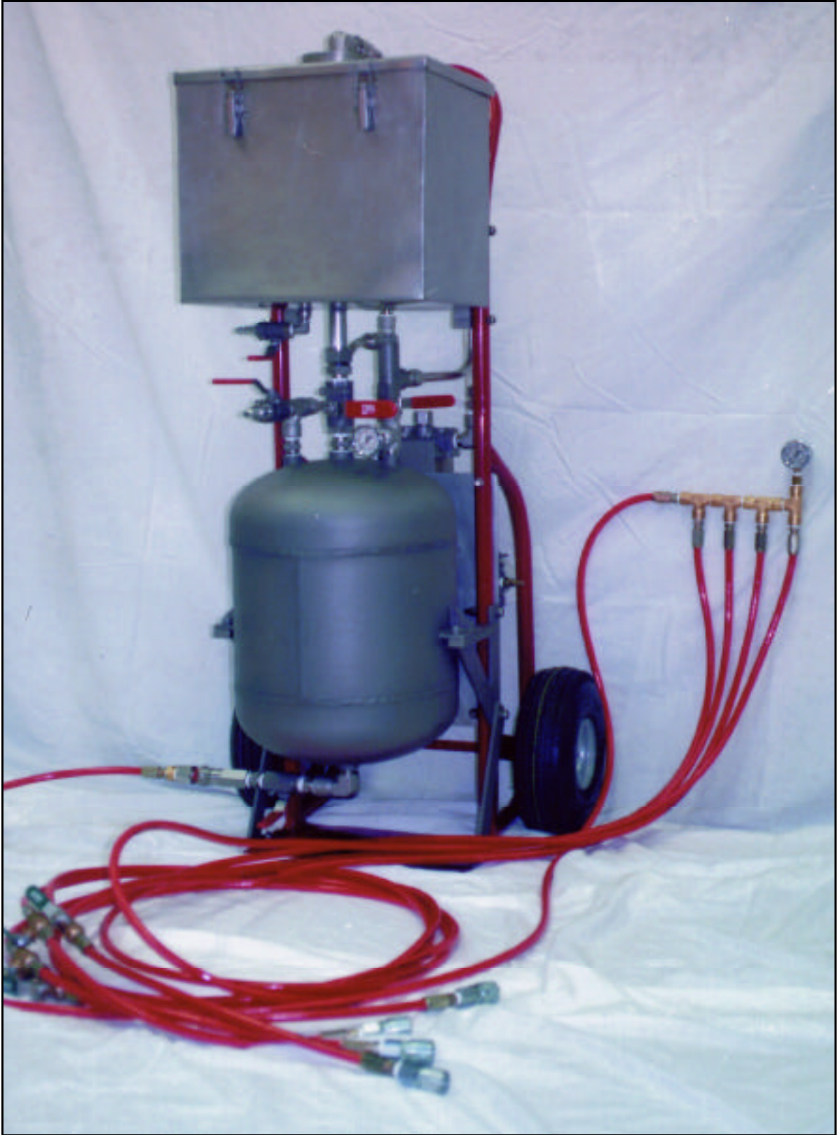
BCP Solvent Cart shown with high pressure solvent manifold attached to pressure tank.
