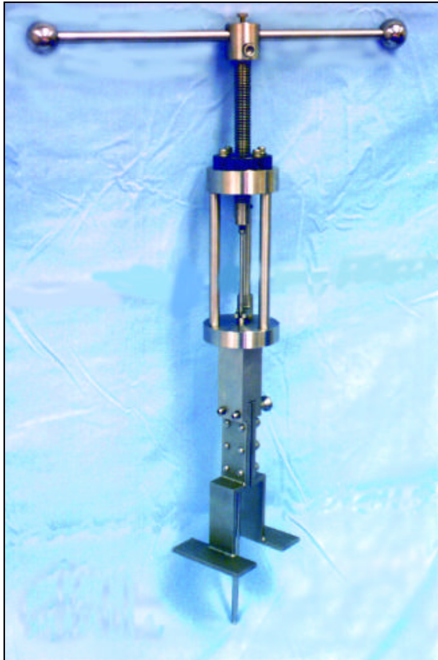
This full length view of the Expansion Tooling shows the thimble clamp that sits on the Seal Table and the screw arrangement that presses the mandrel into the thimble bore.
